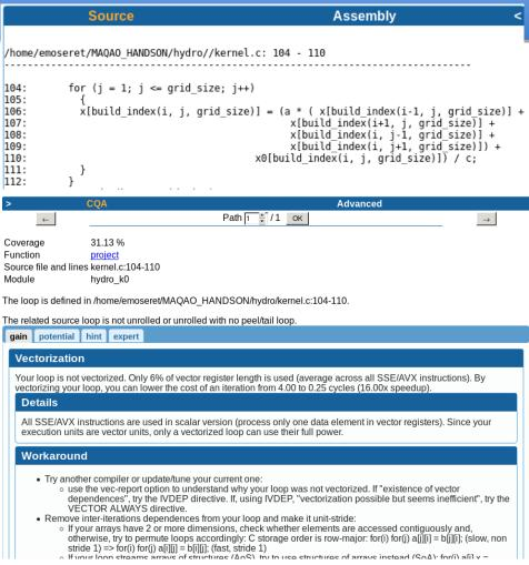
The kernel routine, linearSolver, were inlined in caller functions. Moreover, there is direct mapping between source and binary loop. Consequently the 4 hot loops are identical and only one need analysis.
